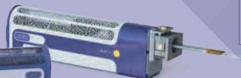
Unity: The world's first Backscattered Electron and X-ray (BEX) Imaging detector
